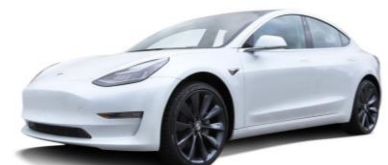
Tesla Model 3, NCA Pack density: ~160 Wh/kg
