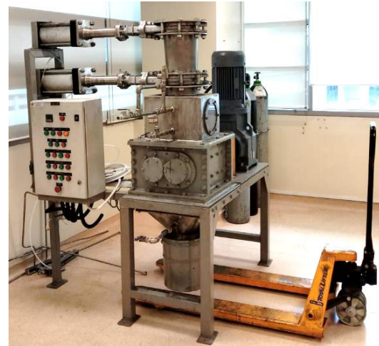
Mechanical Shredder for batteries (10kg/h)
