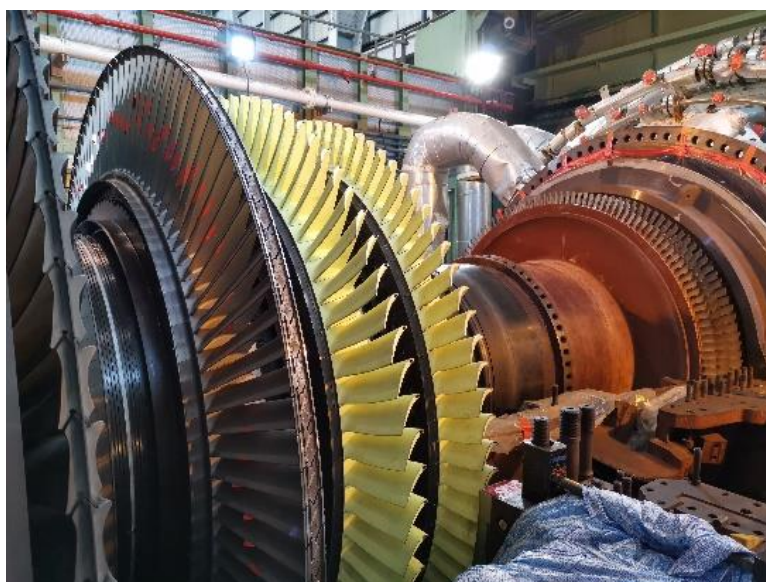
One of the gas turbines which Senoko Energy has upgraded with new cooling technologies and advanced materials, such as thickened thermal barrier coating on the turbine blades (in yellow).
