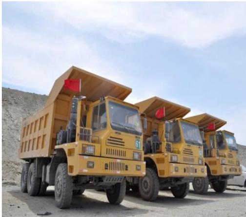
**3 trucks running in coal mine, Xinjiang province. The rate of methanol substituted for diesel 38%, the ratio of methanol to replace diesel at 1.3 within the range of diesel substitution.**
