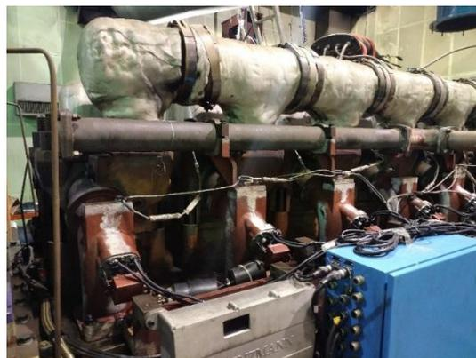
**The engine has two electronic control systems, one for baseline engine, the other for methanol. They can communicate with each other through CAN.**
