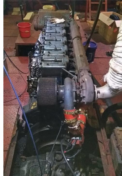
Engine: Weichai 6160, 184kW/1000 rpm. Engine power remains unchanged
