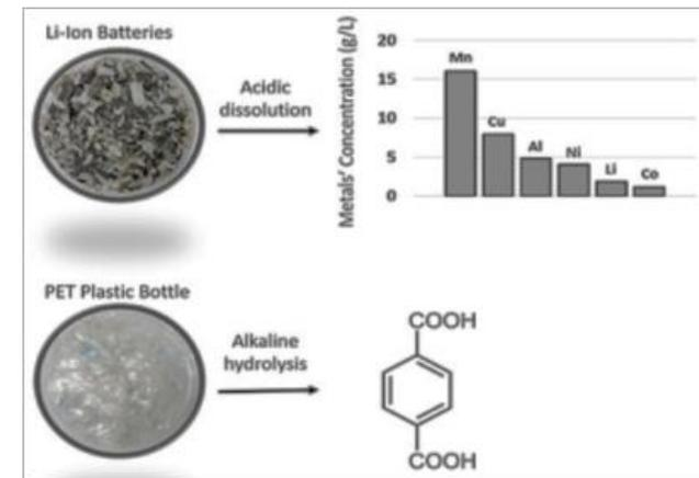
Poly(ethylene terephthalate) from plastic bottles was depolymerized to produce an organic ligand source (terephthalate), and Li-ion batteries were dissolved as a source of metals. By mixing both dissolution solutions together, selective precipitation of an Al-based MOF, known as MIL-53 in the literature, was observed
