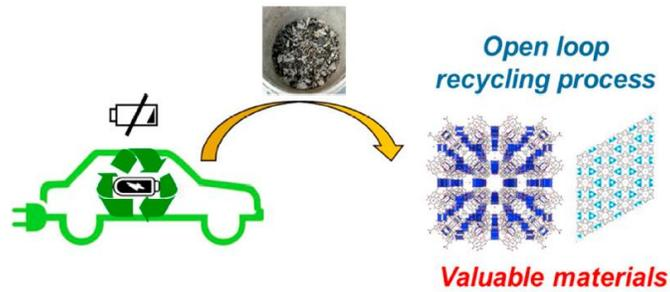
This method shows promising results at the lab scale (15 g of wastes can be converted in 10 g of MOFs) and opens interesting perspectives for the scaled-up production of MOFs.
