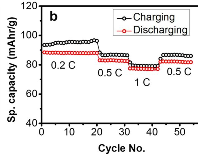
Electrochemical properties of as synthesized LFP, a) Charge discharge curve at 0.2 C current, (inset CV curve) b) cycling at different C.
