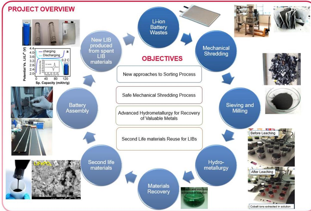
Circular economy process for lithium ion batteries established at NTU
