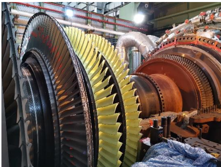
One of the gas turbines which Senoko Energy has upgraded with new cooling technologies and advanced materials, such as thickened thermal barrier coating on the turbine blades (in yellow).
