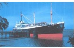
First LNG carrier with 5,000 DWT to bring LNG from US to UK (Methane Pioneer)
